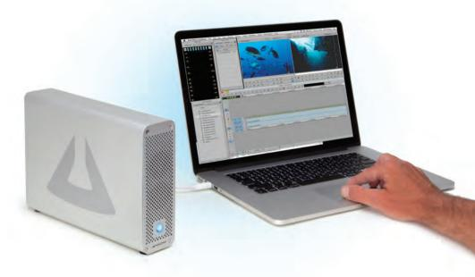
ExpressBox 1T does not have ON/OFF switch. The BLUE LED on the front is an INDICATOR, not a power SWITCH. To turn ON the expansion chassis, connect to a Thunderbolt equipped computer.
