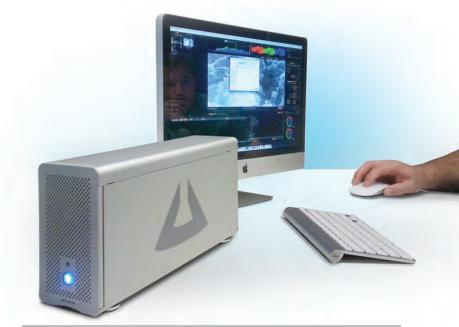
**Note:** ExpressBox 3T does not have ON/OFF switch. The BLUE LED on the front is an INDICATOR, not a power switch. To turn ON the expansion chassis, simply connect to a Thunderbolt equipped computer.
