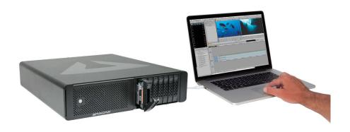
The ROBEN-3 does not have ON/OFF switch. The WHITE LED on the front is an INDICATOR, not a power SWITCH. To turn ON the expansion chassis, connect to a Thunderbolt equipped computer.
