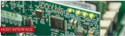
Turn on the host computer. Upon powering up the computer all four Solid Green LEDs on expansion interface cards and Host Interface cards are illuminated.
