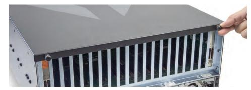
Remove top cover. Loosen the 2 thumbscrews that retain the top cover of the chassis. Slide the cover backwards and upwards.
