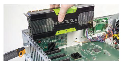
Remove filler bracket for the expansion slot you wish to use in the chassis. Install PCI Express card into the slot connector and secure with retaining screw.
