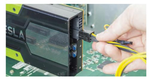
Connect Auxiliary power cables (supplied) as required by the PCle card. High power GPUs typically require one or possibly two (e.g. Tesla K40) PCI AUX power connections. Check with the PCIe card documentation.
