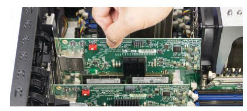
Install the two Magma PCle host interface cards into an available PCl Express slot in the host computer. Use available x16 PCle slot. Secure it with retaining screw.
