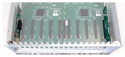
Install the two Magma PCle expansion interface cards in the expansion unit. Install the first Expansion Interface card in the designated PCle "SLOT 0-UPLINK". And install the other Expansion Interface card on PCle "Slot 5-UPLINK. Secure the edge connector bracket with retaining screw.
