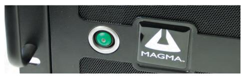
Press the Power Button on the front switch to power up the EB3600 unit. Turn power to the Magma chassis first before powering ON the host computer.
