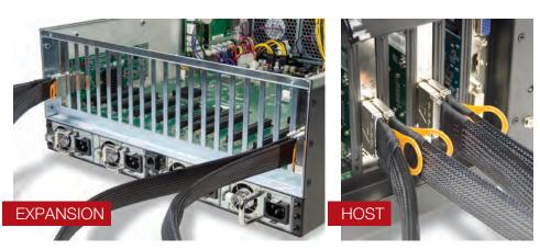
Connect Cables to the back of Expansion Interface cards. And connect the other end of the cable to Host Interface card. Connect Cable from port A of Expansion card to port A of Host card. And from Port B of Expansion to Port B of Host card.
