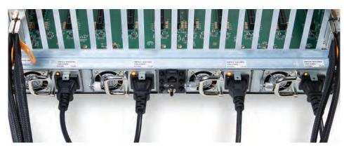
Plug-in all four power cords to the expansion chassis. When using four 110v power cords it is highly recommended to connect them into two separate 110v electrical outlets on different circuit lines to prevent electrical overloads.
