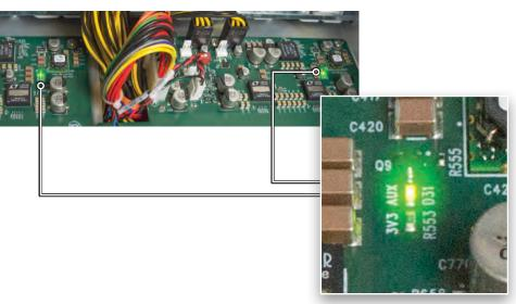
Three Solid Green and One Amber LEDs are illuminated on the expansion interface card LEDs D7,D8 and D3 when on (Solid Green): POWER / 3.3V is good. LED D5, when on (Solid Amber): PCle reset is asserted.
