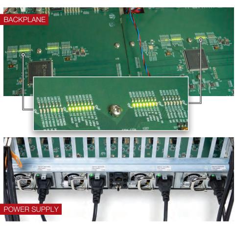
Upon powering on the unit 15 Solid Green LEDs (on each backplane) are illuminated. And power supply LED turns from Amber to Solid Green.
